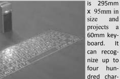
x 95mm in and projects a 60mm keycan recognize up to hundred characters per minute. It is also portable. It can even fit in your pocket. Computers, PDA's, and mobile phones can use the laser keyboard. It is powered by lithium-ion batteries and has more than 120 minutes of continuous typing in its capacity. Even though this gadget is small, it is still a remarkable piece of technology.
